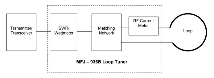
Figure 6 Typical MFJ-936B *Loop Tuner*<sup>™</sup> Configuration
